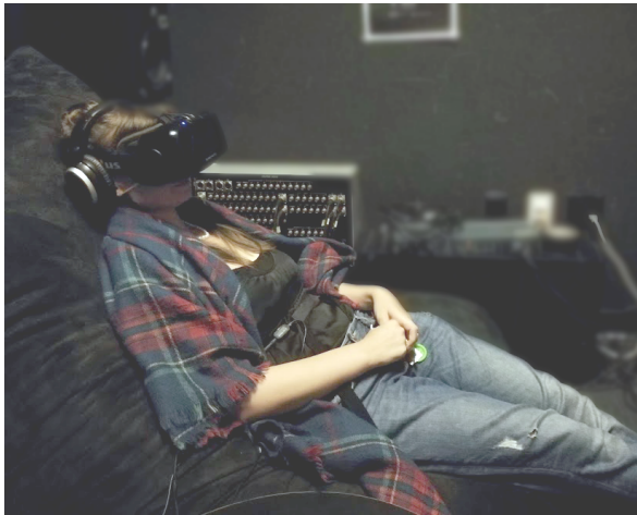
Figure 3. The participant interacting with the VE, wearing breathing sensors, headphones, and Oculus Rift while seated on the cushion
