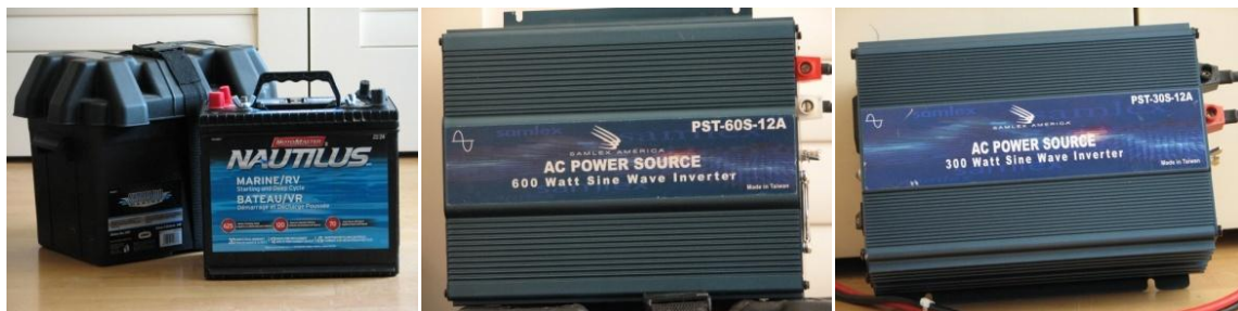
Figure 4.3. Marine batteries and 300 W and 600 W pure sine wave inverters from Module 2 Extended Power system of LocoMotoArt
